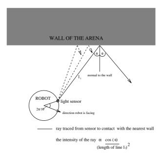
Figure 7: The rays are projected from the light sensor and the intensity registered is a a product of their first encounter with an object (the automaton or a wall).
