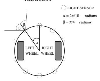
Figure 3: The Simulated Robot
