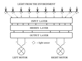
Figure 4: Converting Light Intensities to the Robot's Movement
